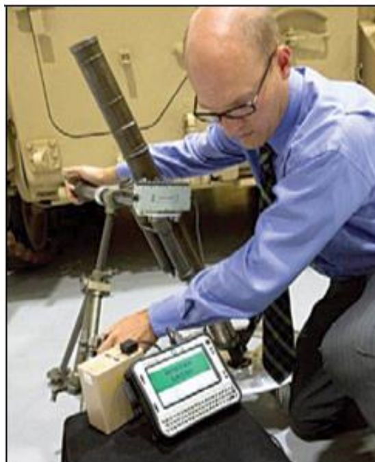
Weaponized Universal Lightweight fire Control WULF (US Army).
